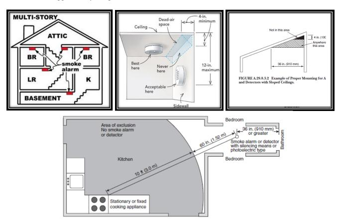
FIGURE A.29.8.3.4(4)(b) Example of Smoke Alarm or Smoke Detector Placement Between 10 ft (3.0 m) and 20 ft (6.1 m) Away in Hallway from Center of Stationary or Fixed Cooking Appliance.
